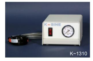
**K~1310 Gas Flow Control:** The operator, by means of an on/off footswitch, releases the gas to the work area. Immediately after the scrub cycle stops, the footswitch is activated and the die is showered with cool forming gas. A manual adjustment is provided to meter the amount of gas to be released.
