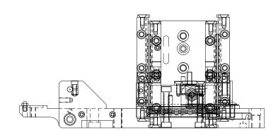
It should be understood that the pneumatic axis brakes cannot prevent deliberate efforts at movement, but that they are a significant aid in maintaining correct tool to work contact during bonding.
